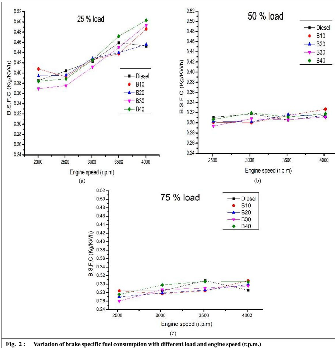
Fig. 2 : Variation of brake specific fuel consumption with different load and engine speed (r.p.m.)
