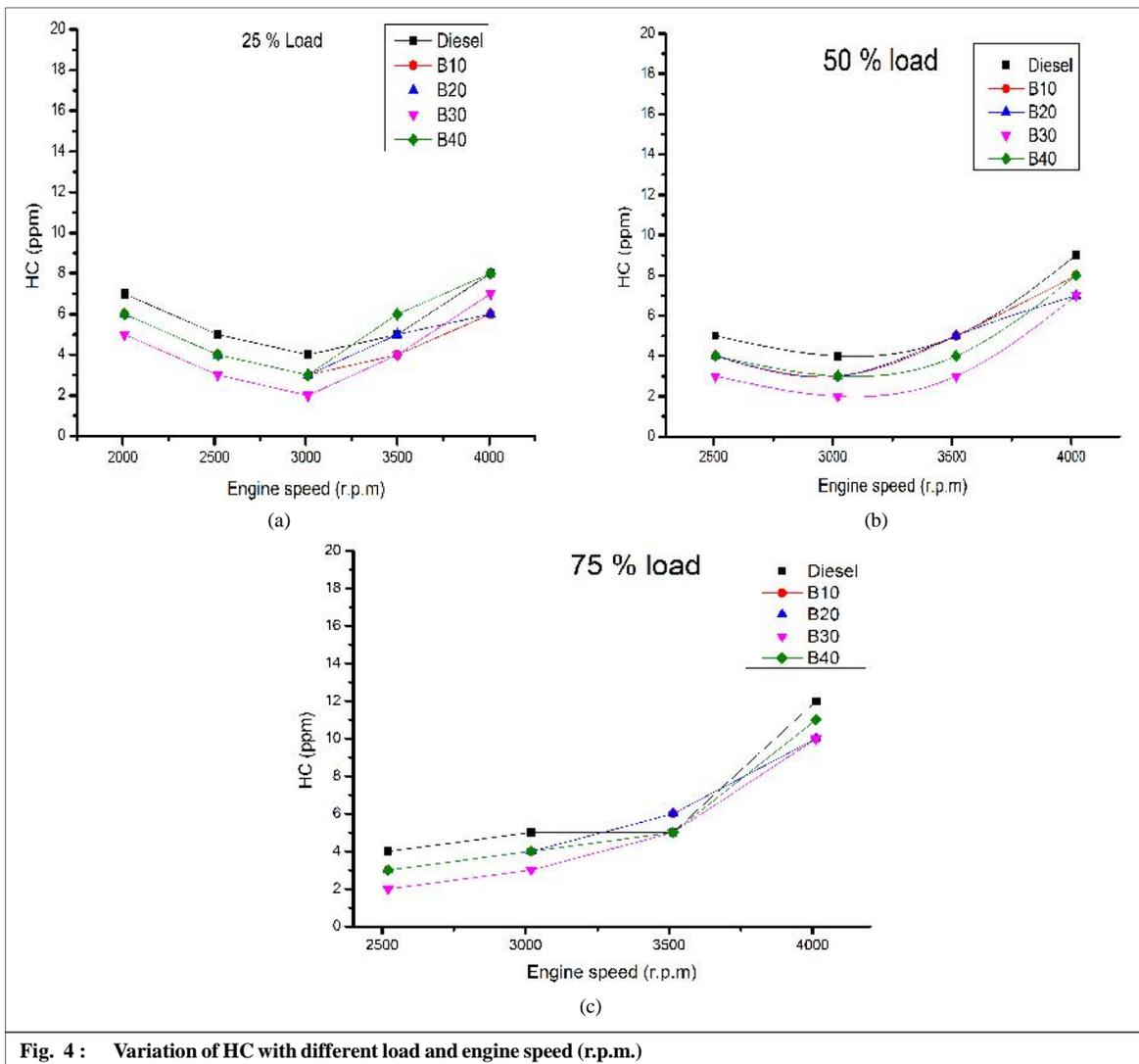
Fig. 4 : Variation of HC with different load and engine speed (r.p.m.)
