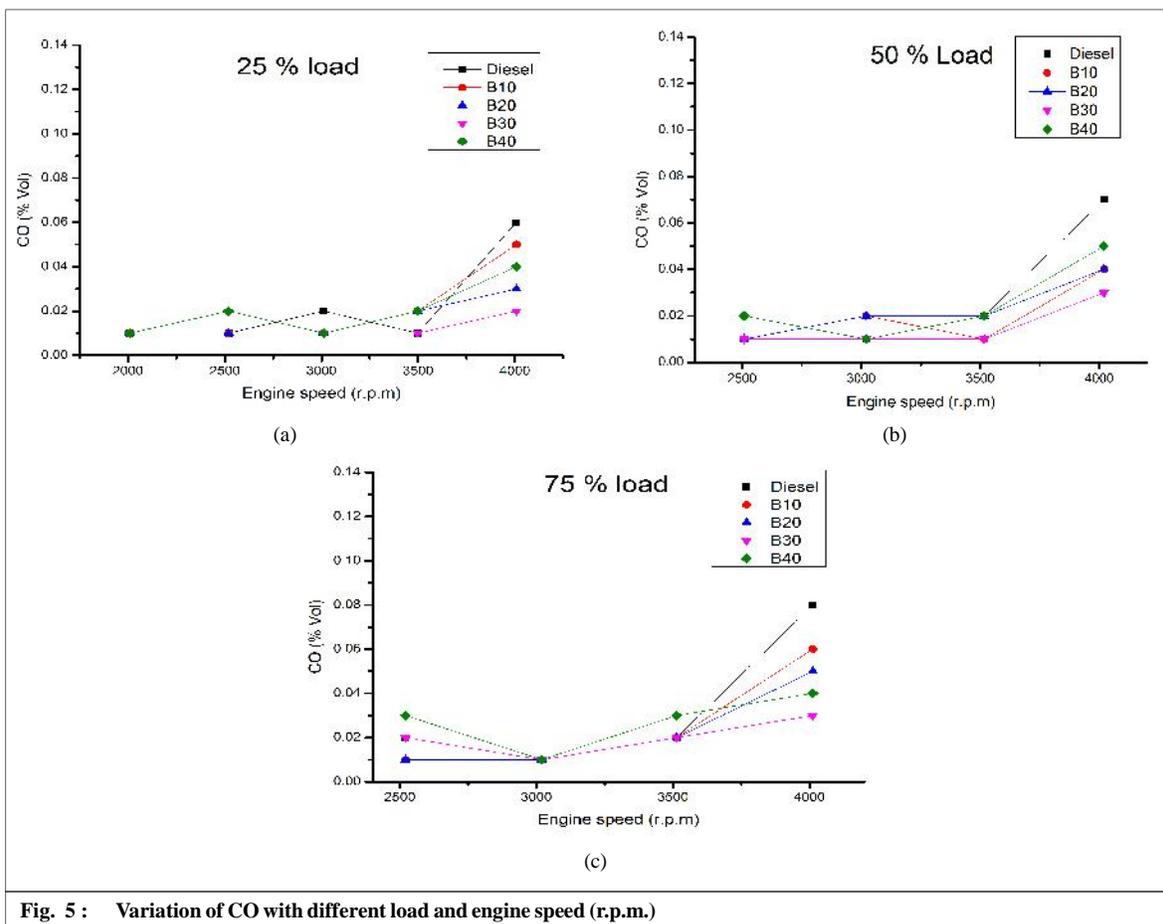
Fig. 5 : Variation of CO with different load and engine speed (r.p.m.)
