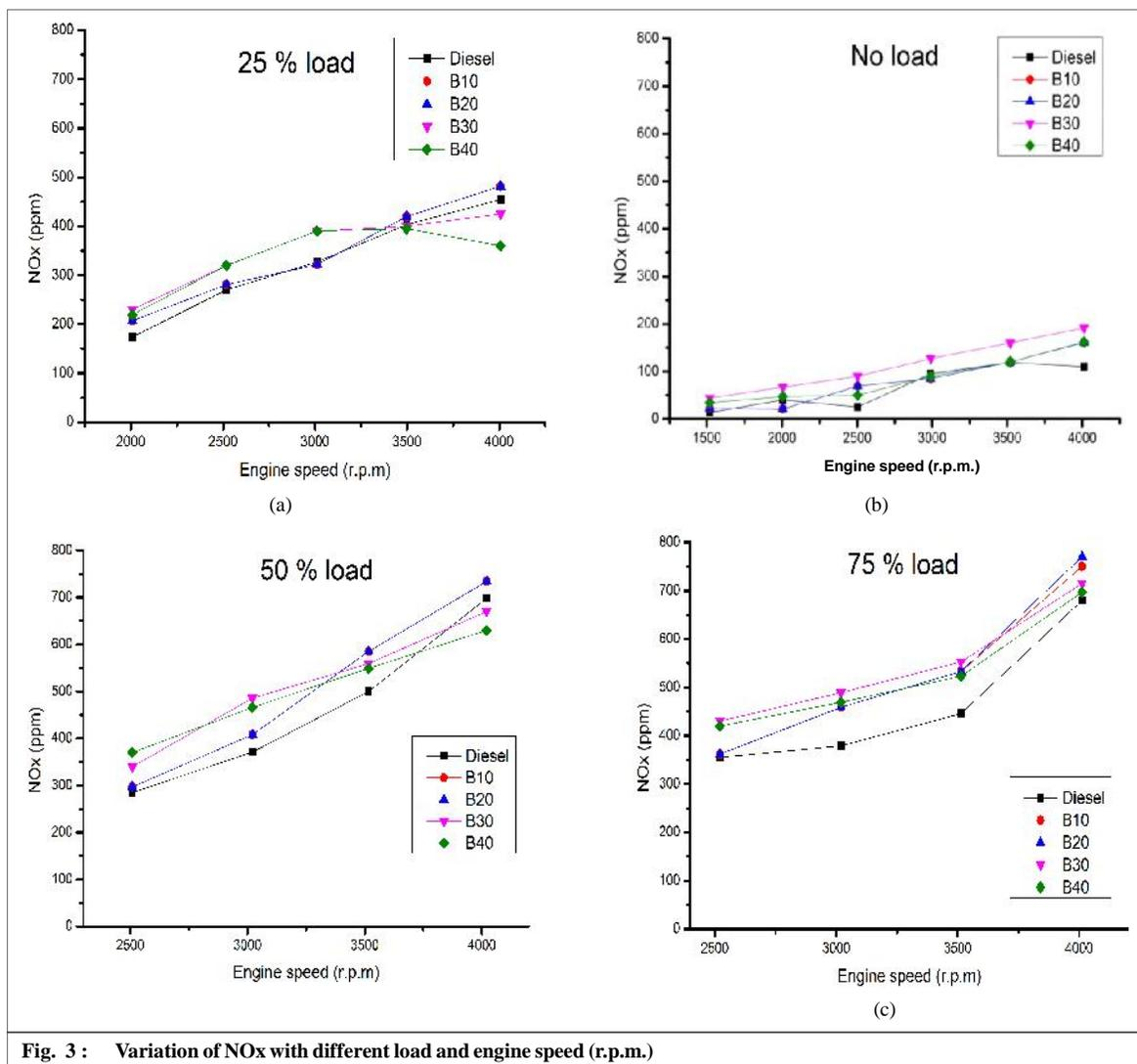
Fig. 3 : Variation of NO<sub>x</sub> with different load and engine speed (r.p.m.)
