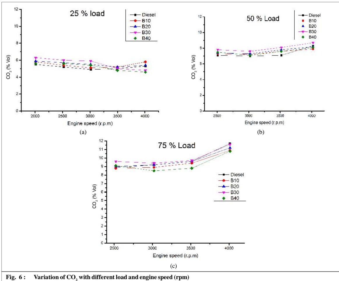
Fig. 6 : Variation of CO<sub>2</sub> with different load and engine speed (rpm)
