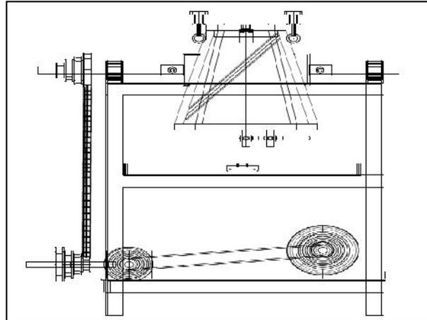
Fig. A : Auto-cad diagram of improved butter churn
