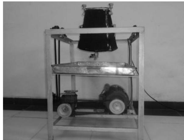
Fig. B : Skid mounted improved butter churn
