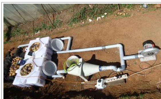
Fig. B : Ventilation of evaporative cooled air and atmospheric air
