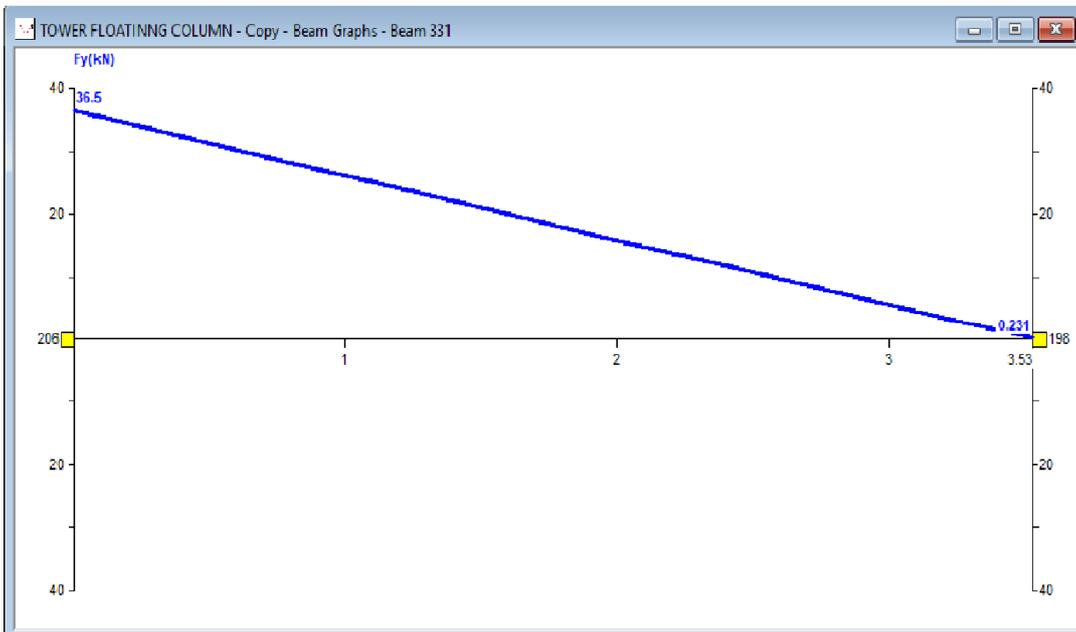
GRAPH: - 5.7 MAXIMUM SHEAR FORCE IN BEAM FOR BUILDING HAVING FLOATING COLUMNS
