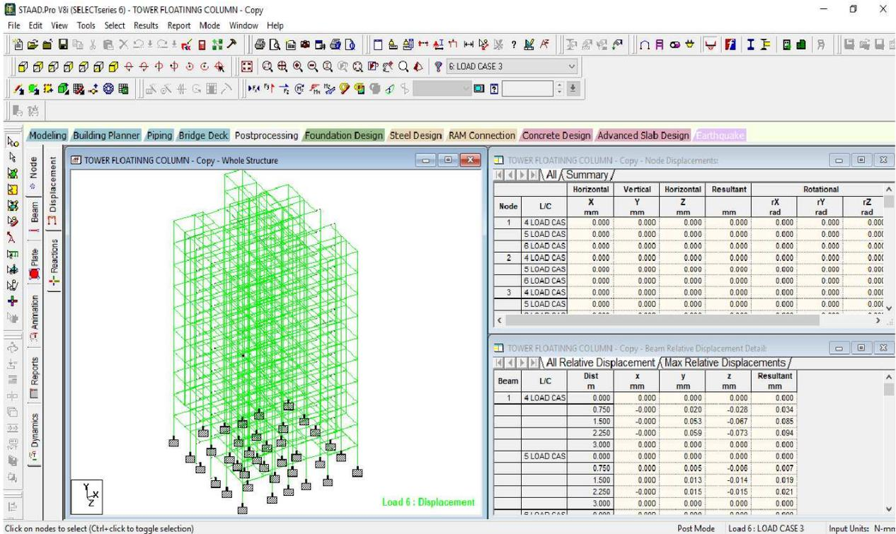
**Fig.5.6 – STAAD Pro Model showing Nodal displacement in Building without floating columns**
